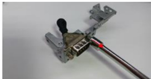
14: Desparafusar e remover porta DB9.
