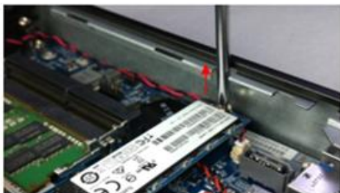
11: Conectar SSD e parafusar. PN.: 22232200351 – 1
