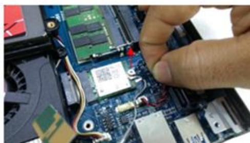
16: Desconectar antenas auxiliar, e principal na placa wireless.
