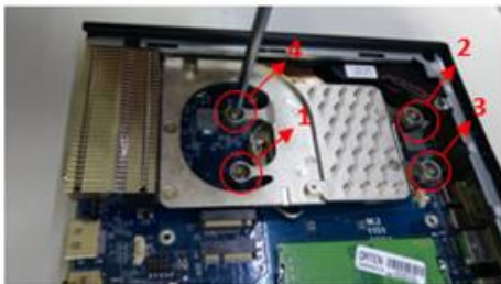
18: Desconectar, desparafusar, e remover cooler.
