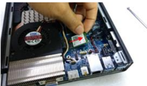
17: Desparafusar e remover placa de wireless.
